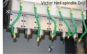
8-month run-in period after repeated tests and adjustment before the quad-spindle took the full speed in the operation, but all that effort have well been paid by a guaranteed precision process with multiplied productivity.
